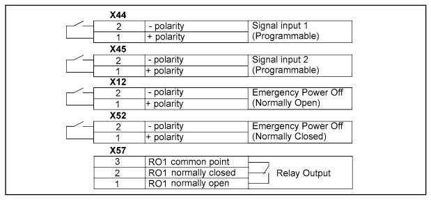
Figure 11 External control cable connections to the UPS.
