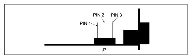
**Figure 28** XSlot Hot Sync card and jumper settings: Resistor ON: PIN 1 and PIN 2 connected, No resistor: PIN 2 and PIN 3 connected (default setting).
