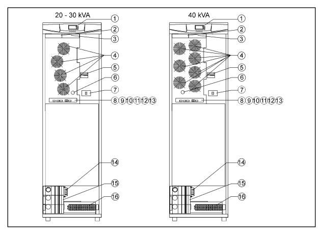
**Figure 5** Powerware 9355 20-30 kVA and 40 kVA layout: 1:Graphical LCD; 2:XSlot-1; 3:XSlot-2; 4:Fans; 5:Input (rectifier) breaker (20-30 kVA)/switch (40 kVA); 6:Battery start button; 7:Battery breaker; 8-13: Connectivity terminals; 14:Ground terminal; 15:MBS; 16:Power cable terminals
