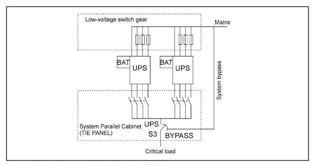
Figure 29. System bypass switch of the optional SPM
