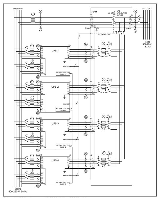
Figure 24 Wiring diagram with SPM-30-4 and SPM-40-4
