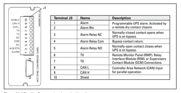
Figure 26 XSlot Hot Sync card and terminal interface
