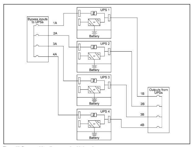
Figure 25 Bypass wiring diagram and cable length notes
