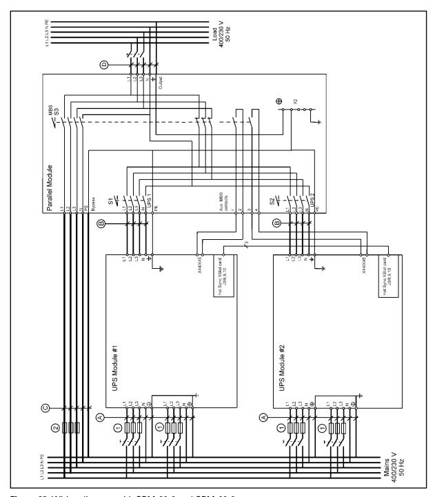
Figure 23 Wiring diagram with SPM-30-2 and SPM-60-2
