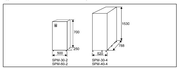
Figure 20 Dimensions of the SPM-30-2 and SPM-60-2, SPM-30-4 and SPM-40-4
