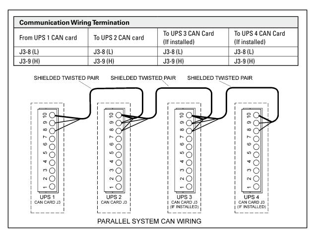
Figure 27 Communication cabling wiring
