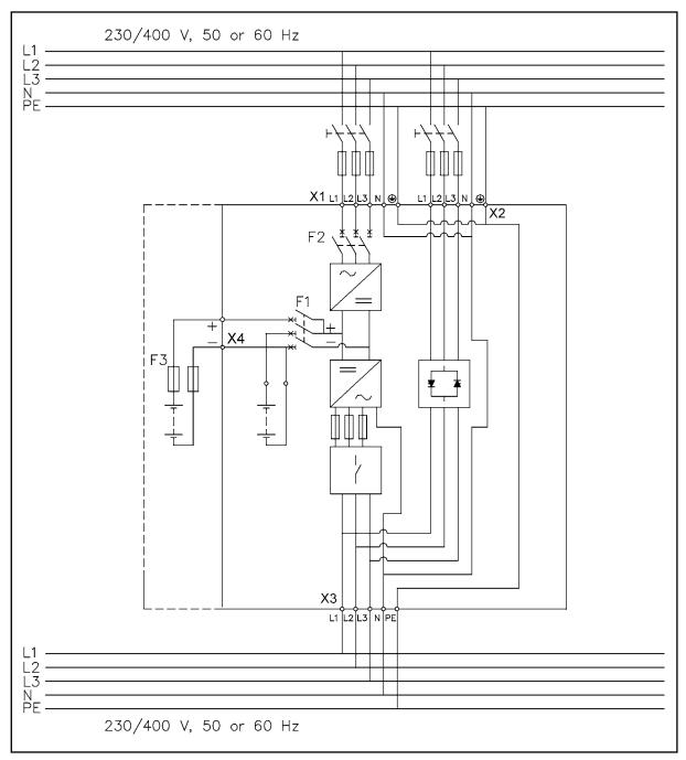
Figure 8 Wiring diagram of UPS N-model.
