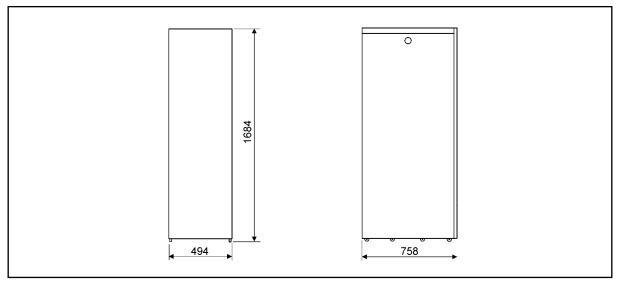
Figure 31 Dimensions of the External Battery Cabinet
