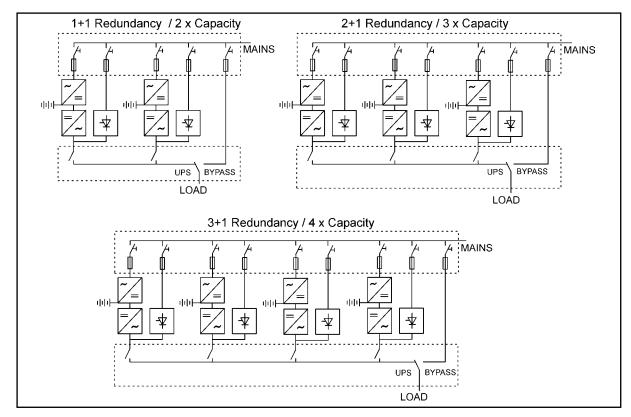
Figure 19 Parallel configurations with UPS modules.
