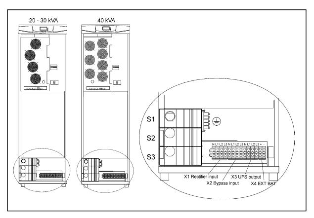
**Figure 6** Location of the power terminals. S1:Service Bypass Switch; S2:Static Bypass Input Switch; S3:UPS Output Switch. Disconnect all internal battery strings before operating with the terminal X4.
