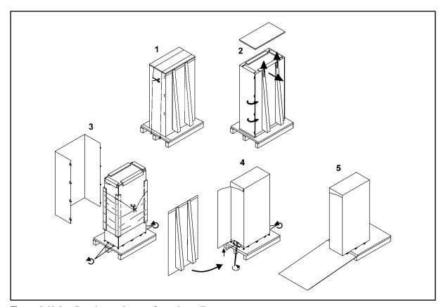
Figure 3 Unloading the equipment from the pallet.
