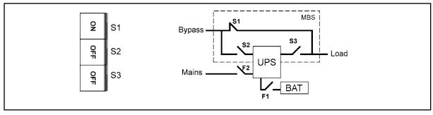
Figure 18 The service (bypass supplying the load) positions of the three MBS switches.
