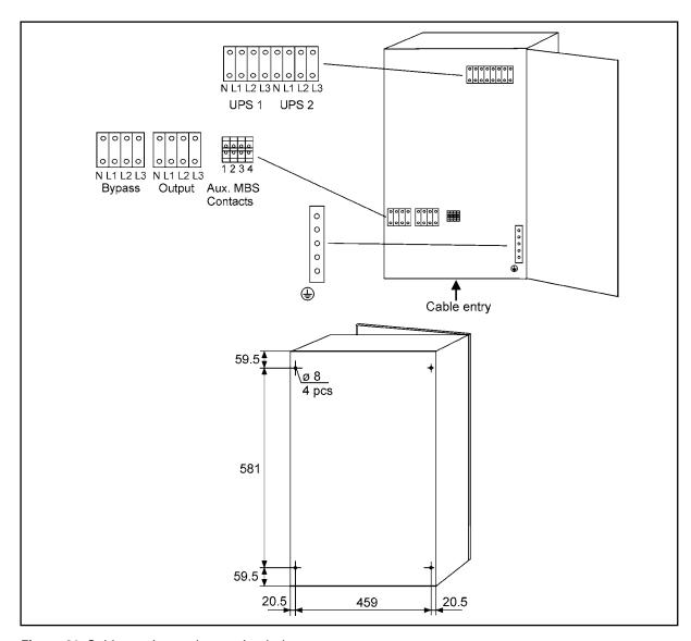
Figure 21 Cable routing and mounting holes
