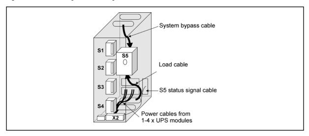
Figure 22 Cable routing of SPM-30-4 and SPM-40-4 cabinets
